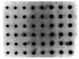
Figure 2. Photomicrograph of 4:1 real-time spot area modulation: 300 dpi with every fourth pixel printed; 3,000 lines/second
