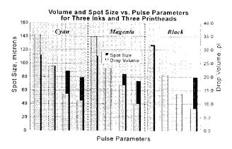
Figure 1. Example of drop volume and spot size modulation results obtained with three ink/printhead combinations
