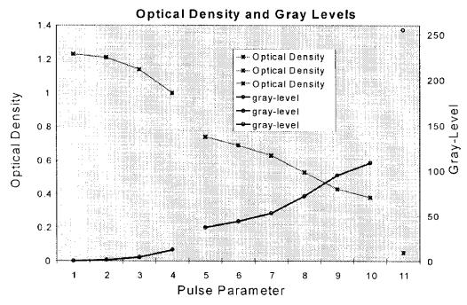
Figure 3. Optical density range and grey-level assignment resulting from drop volume modulation.
